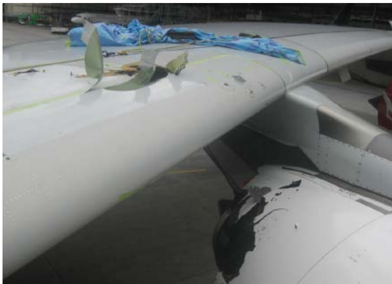
Figure 8: Wing damage caused by engine failure
