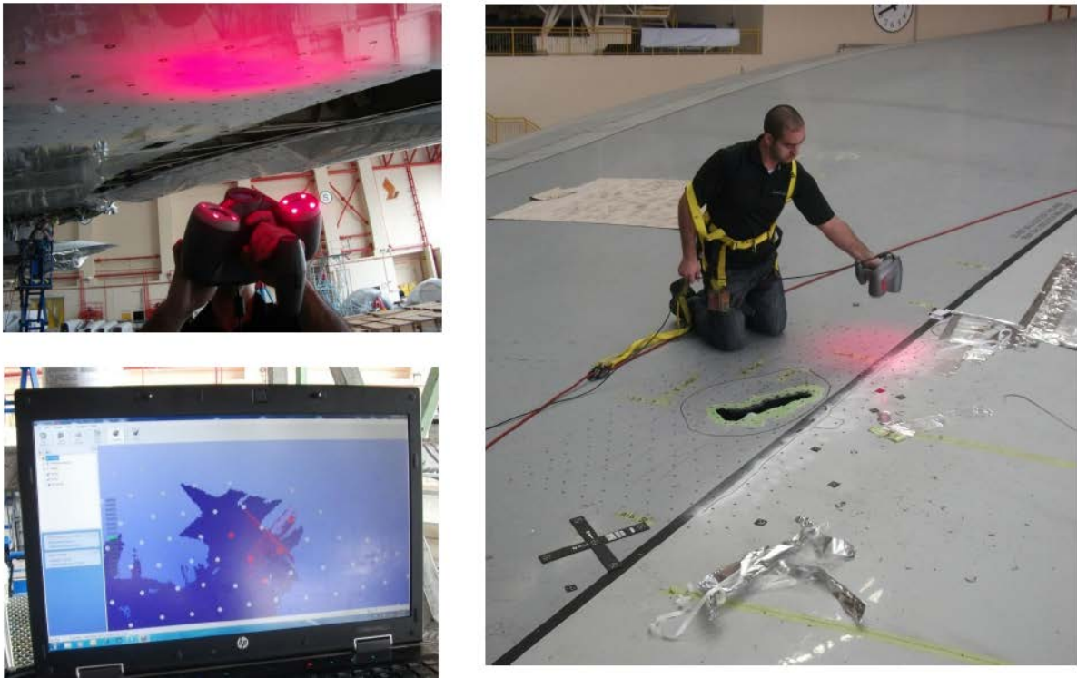
Figure 9: Inspector scanning the damaged wing section with the laser scanner
