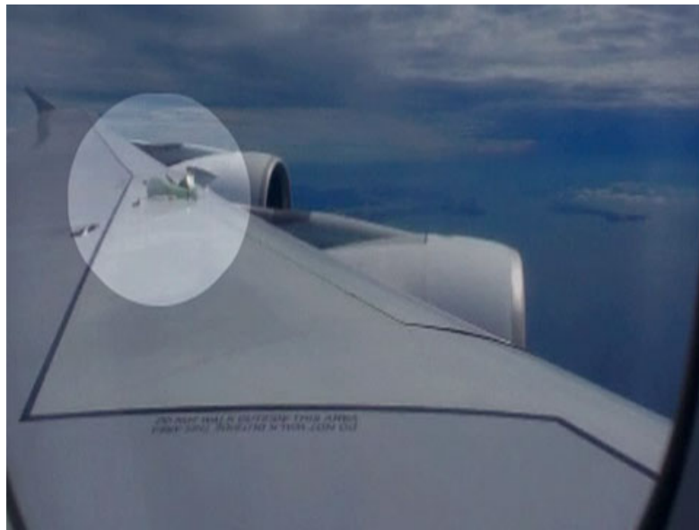
Figure 7: Picture of wing damage during flight
